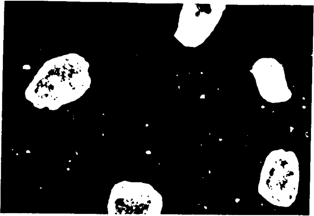
PLATE (3.9) MICROSCOPIC VIEW OF THE EXPERIMENTAL SAND [ d_{50} = 0.15\text{mm} ].
